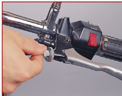
8. Adjust Bowden cable
