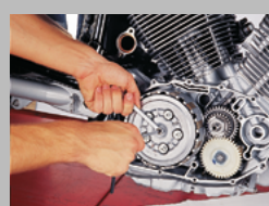
6. Adjust clutch free play at clutch release mechanism, procedure may vary model specific.
