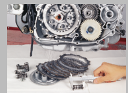
4. Check: free length of springs and wear of steel discs, clutch cage and inner basket. Replace parts if required.
