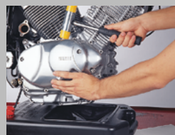
2. Dismantle screws stepwise, remove clutch case cover, clean sealing surface, pay attention to fitting sleeves
