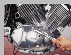
7. Remount clutch case cover using new gasket, pay attention to fitting sleeves, tighten screws stepwise.
