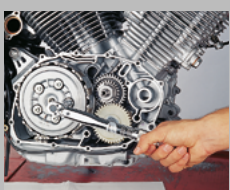
5. Start reassembly with friction disc, tighten screws at clutch pressure plate stepwise.
