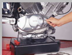
1. Prepare required tools, cover floor, drain oil.
