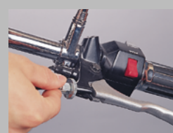
8. Adjust Bowden cable to 4mm free play.
