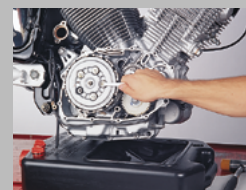
3. Remove clutch pressure plate and clutch discs. Assort in correct mounting sequence.
