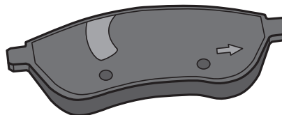
Brake pad with recess and details of the fitting direction on the back plate of the pad
