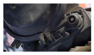
Turn the adjuster clockwise until the pads touch the brake disc. Then turn the adjuster back by three to four clicks. Install the cap on the adjuster.
