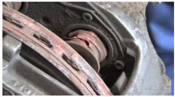
Extend the pistons (tappets) fully using the adjuster and check the bellows for damage.
