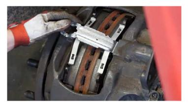
3.4.2 Install the pad retaining bracket
