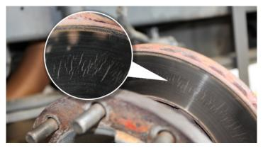
Check the crack pattern on the brake disc.
