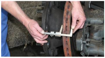
Measure the brake disc at the thinnest location (note the burr on the disc edge).
