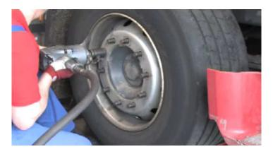
Lift and secure the vehicle. Remove the wheel.
