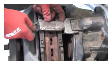
Remove the locking pin, washer and bolt on the pad retaining bracket. Remove the brake pads including retaining bracket and wear contact set.
