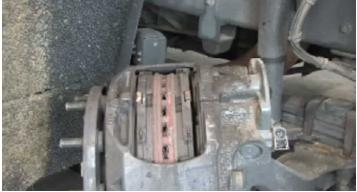
Remove the inner brake pad. Pull the brake caliper towards the outside of the vehicle and remove the outer brake pad.
