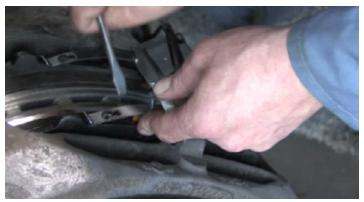
Install the pad retaining bracket, bolt, washer and locking pin.
