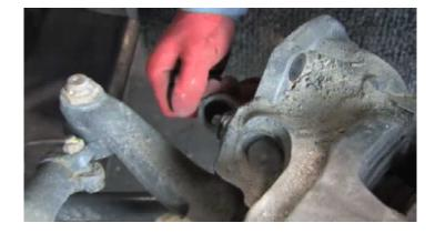
Remove the cap on the adjuster and turn the adapter below anti-clockwise until the pistons (tappets) reveal the inner pad.
