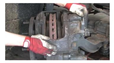
Check correct function of the guide pins by moving the housing back and forth. It has to be possible to move the housing by hand (without tools) across the entire displacement range.
