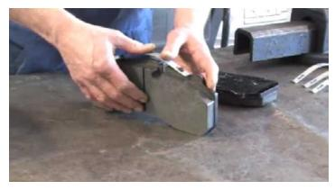
Install the pad retaining springs from the TRW brake pad set on the pads.
