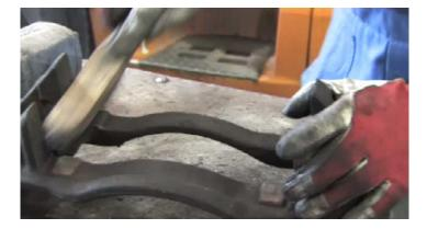
Remove any dirt and traces of corrosion from the contact surface of the brake pads on the brake carrier. Clean the carrier thoroughly with TRW brake cleaner.
