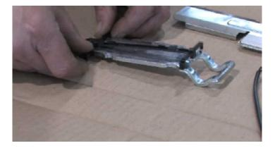
Install the cable guide and the wear contact set on the pad retaining bracket.
