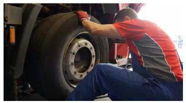
Mount the wheel, centre it and secure it with the tightening torque specified by the vehicle manufacturer.
