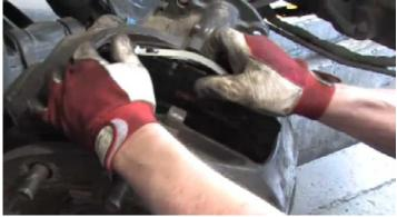
Insert the inner brake pad. Pull the brake caliper towards the outside of the vehicle and insert the outer brake pad.
