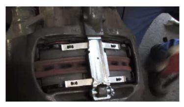
Actuate and release the brake. Turn the brake disc by hand.
