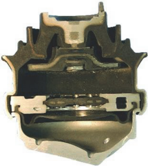
Fig. 3: Original hydraulic part
