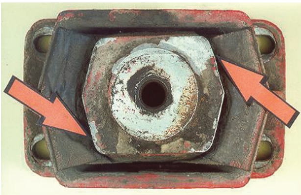
Fig. 2: Wear of a rubber-to-metal component
