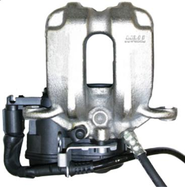
Turn the brake housing until the actuator (motor/gear unit) points downwards. This makes it possible for the enclosed air to get into the piston via the adjusting nut .
