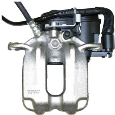
Turn the brake housing until the actuator points upwards. This makes it possible for the air from the piston to get into recess of the bleed hole.
