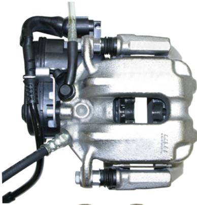
In the installation position, fill and bleed the brake using the bleeder unit (bleed nipple above the piston). After this, completely reduce the brake fluid pressure.
