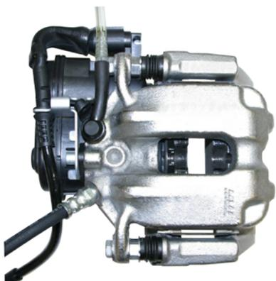
Install the calliper again and fasten it as specified. If required, carry out this procedure with the other brake calliper. Finally, use the bleeder unit to bleed the entire brake as usual.
