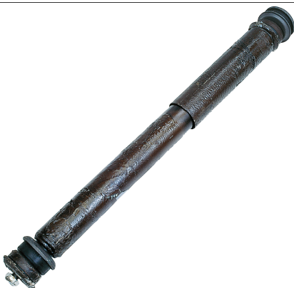
Fig. 3: Undercoat / anti-corrosion wax
