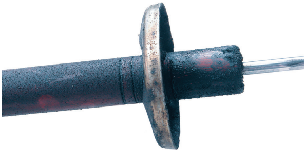
Fig. 1: Oil mist on the shock absorber
