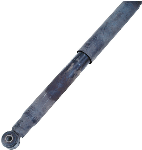
Fig. 1: Oil mist on the shock absorber
