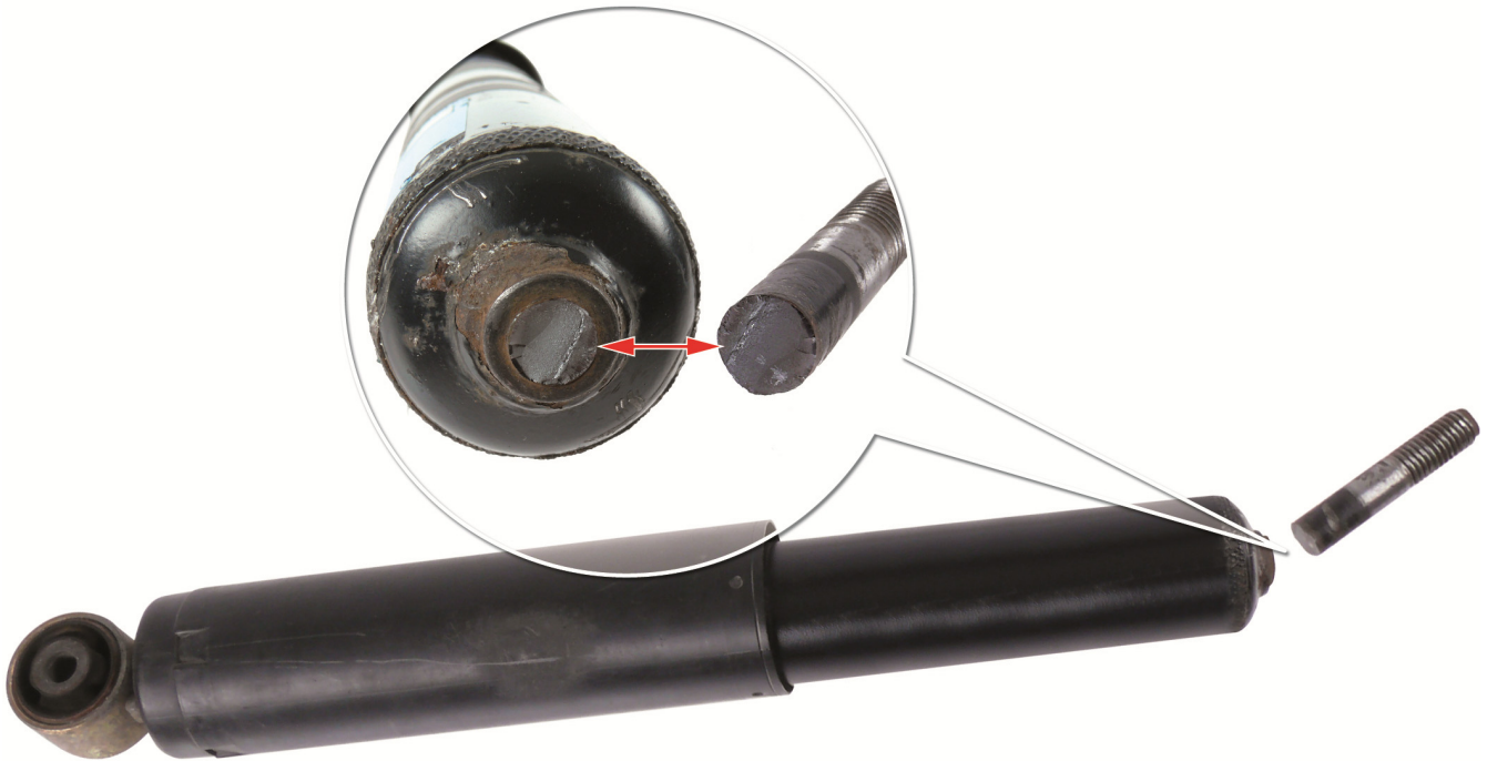
Fig. 1: Pin joint broken due to changing bending strain
