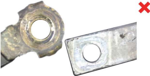
Fig. 1: Ground connection prior to cleaning: Poor connection
