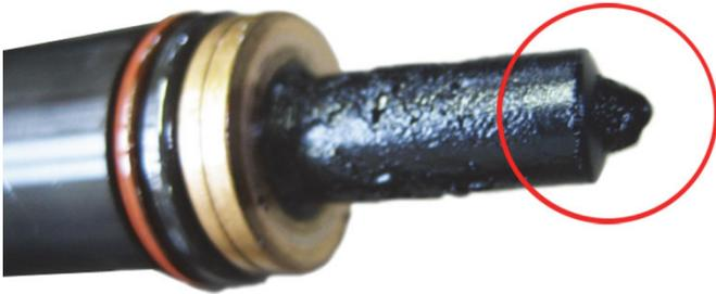
Fig. 3: Unit-injector element coked
