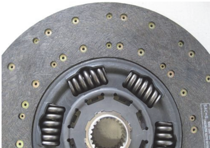
Fig. 3: Lining on the transmission side
