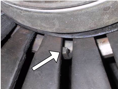
Fig. 1: Incorrect position for the pilot pin on the release collar – the pin has slipped under the diaphragm spring.
