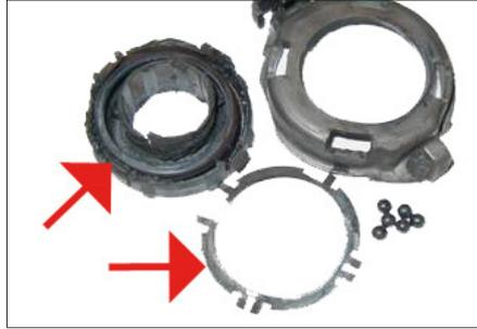
Fig. 4: Mechanical damage and overheating on the release bearing
