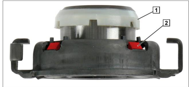
Fig. 2: Release bearing
