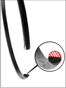
Fig. 3: Worn securing ring
