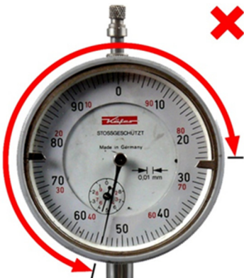
Fig. 3: Lateral run-out \geq 0.5 mm
