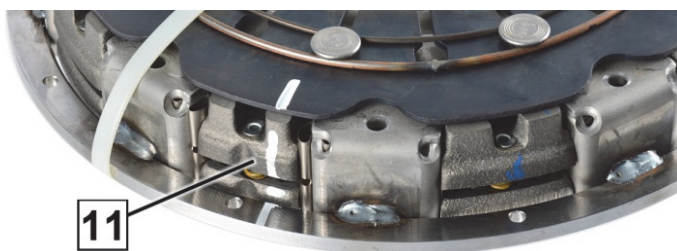
Fig. 6: Marking on the clutch housing
