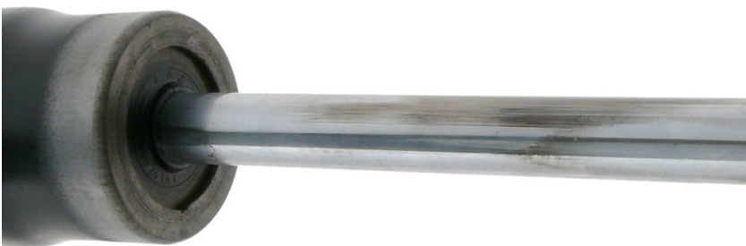
Fig. 2: Chrome layer of the piston rod worn out on one side due to warped installation
