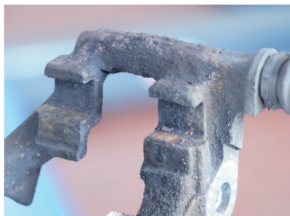
Support d'étrier corrodé
