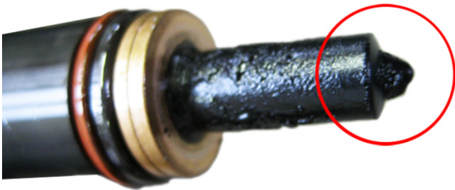
Fig. 3: Unit-injector element coked
